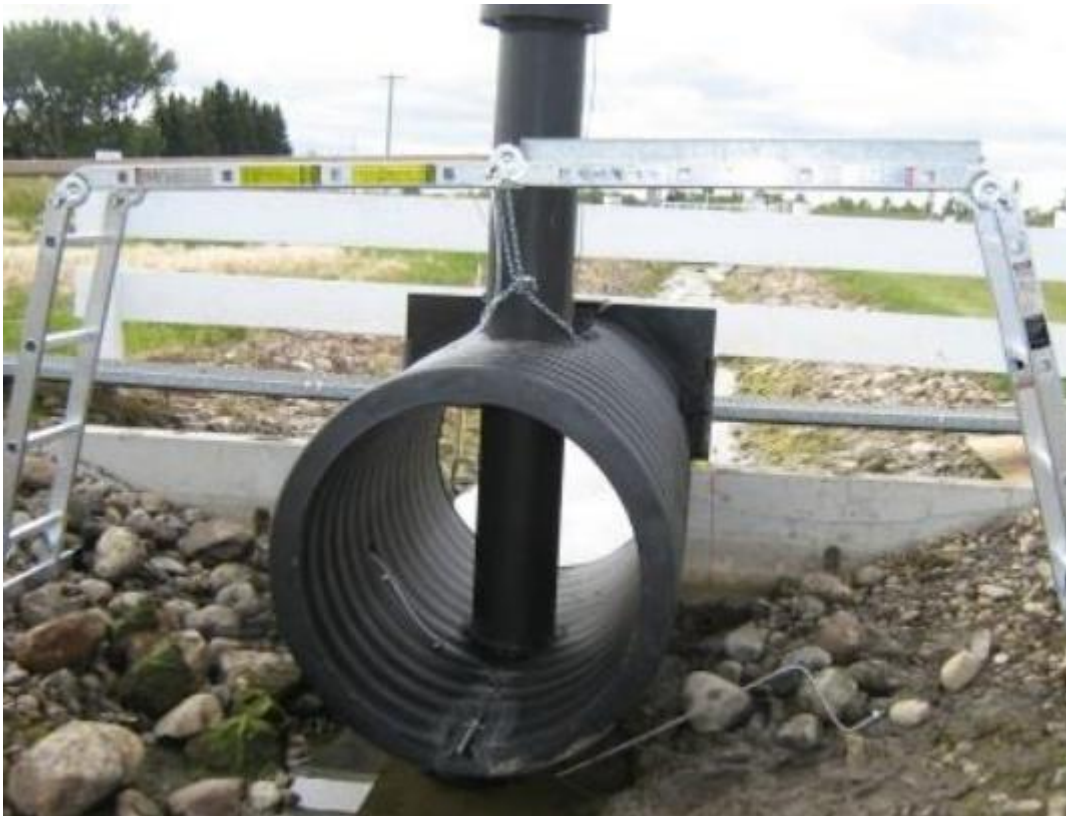
Figure 8. Circular flume in Canada used to measure flow in a canal (Ontkean, 2015).
