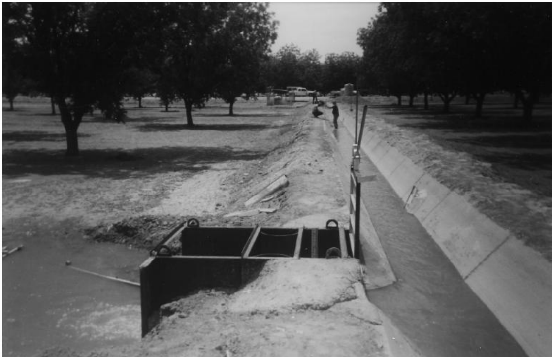
Figure 15. An S-M flume installed in a turnout in a pecan farm in La Union, NM (Samani, 2005).
