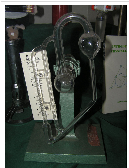
A McLeod gauge, drained of mercury
