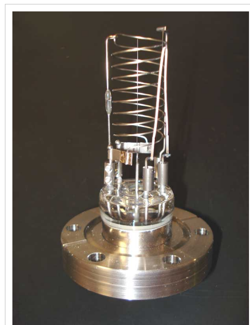
Bayard-Alpert hot cathode ionization gauge
