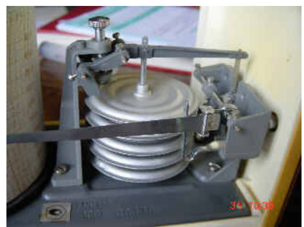
A pile of pressure capsules with corrugated diaphragms in an aneroid barograph.
