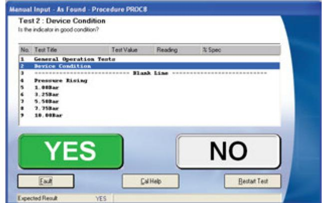
A PASS / FAIL type test allows the general operation to be recorded – simply click on PASS or FAIL to record result.
