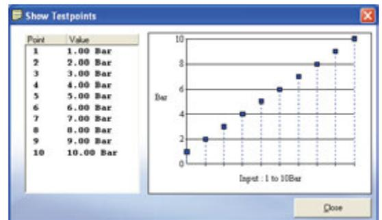
Enter the Low and high pressure range values and the number of test points – once selected the values can be viewed in a graph display by clicking 'Show Test Points'.
