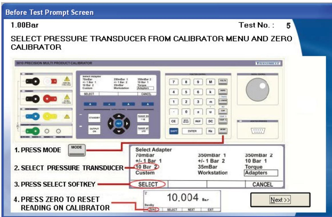
An on-screen prompt shows how to set the calibrator to the require torque mode :
