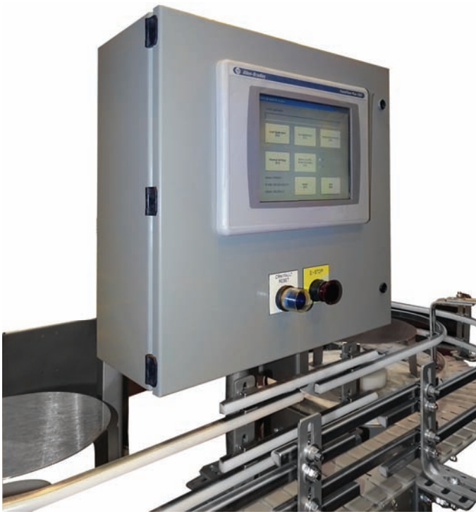
Figure 2-50 Human Machine Interface (HMI). Source: Courtesy of Nercon.
