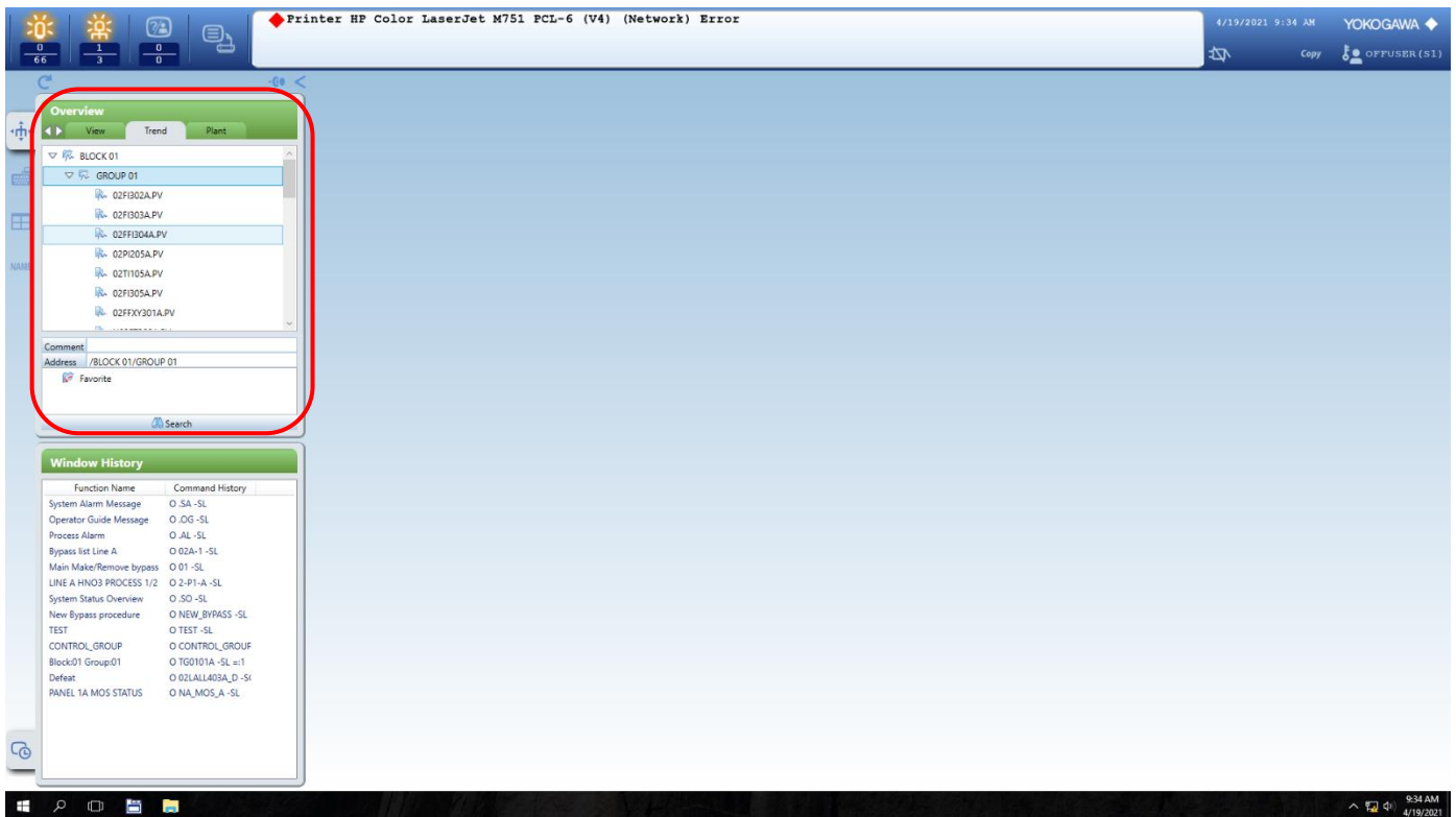
Figure 26: The trend tab in the overview toolbox contains groups of parameters whose trends can be viewed together.
