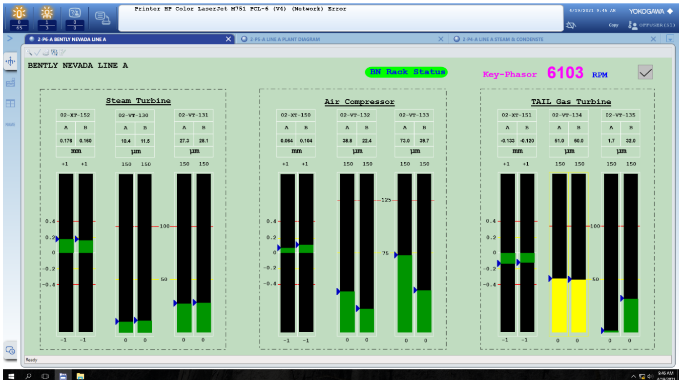
Figure 9: Custom graphic page showing vibrations taken from Bently Nevada BN3500
