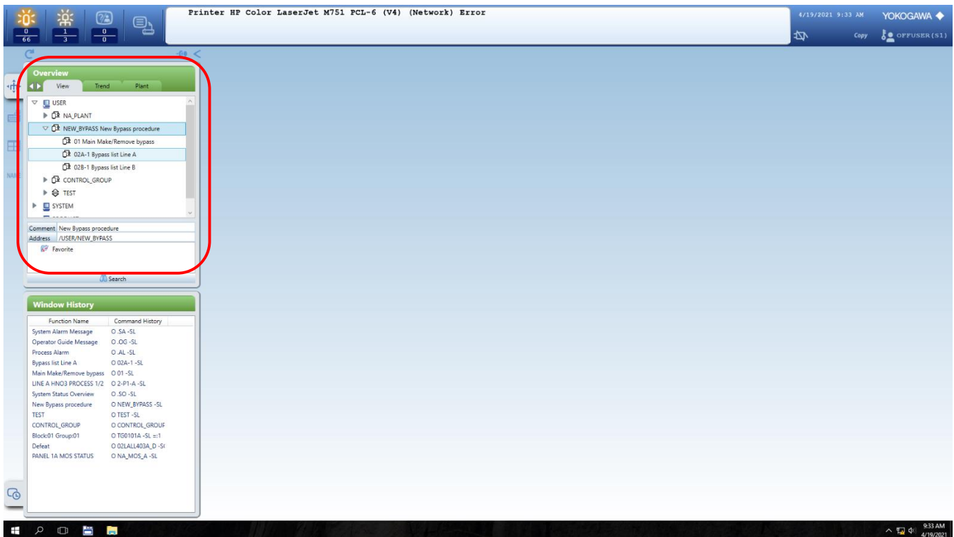
Figure 33: Accessing the make/remove bypass page using the view tab in overview toolbox
