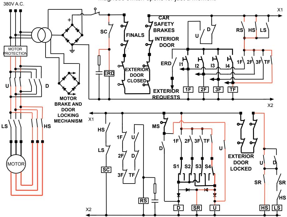
Once the car comes close to the requested floor the direction selector (S4) takes the central position
