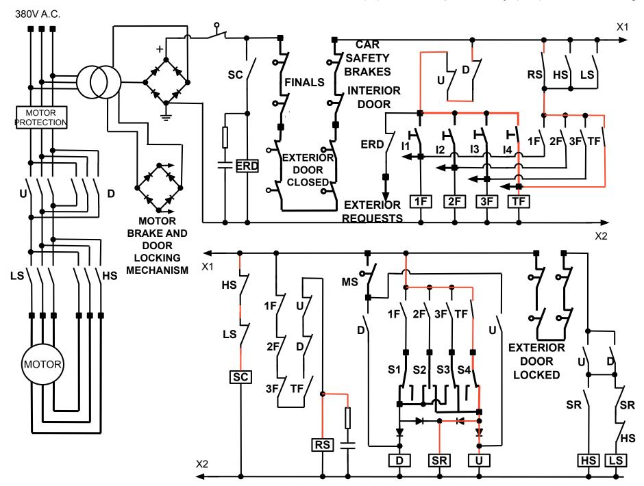
Then the direction contactor (U) and the speed relay (SR) are also energized The reset relay (RS) keeps on for some seconds due to the capacitor
