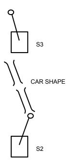
When a request button is pressed the elevator takes the right direction due to the selectors fixed in the shaft on each floor.
