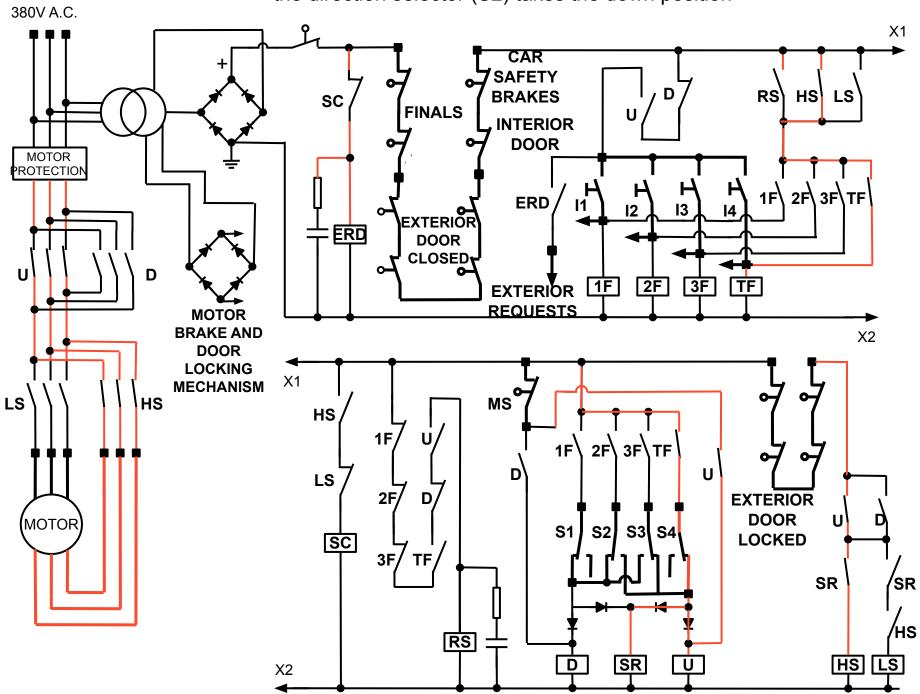
Third floor: the direction selector (S3) takes the down position and the level magnetic switch opens for just a moment
