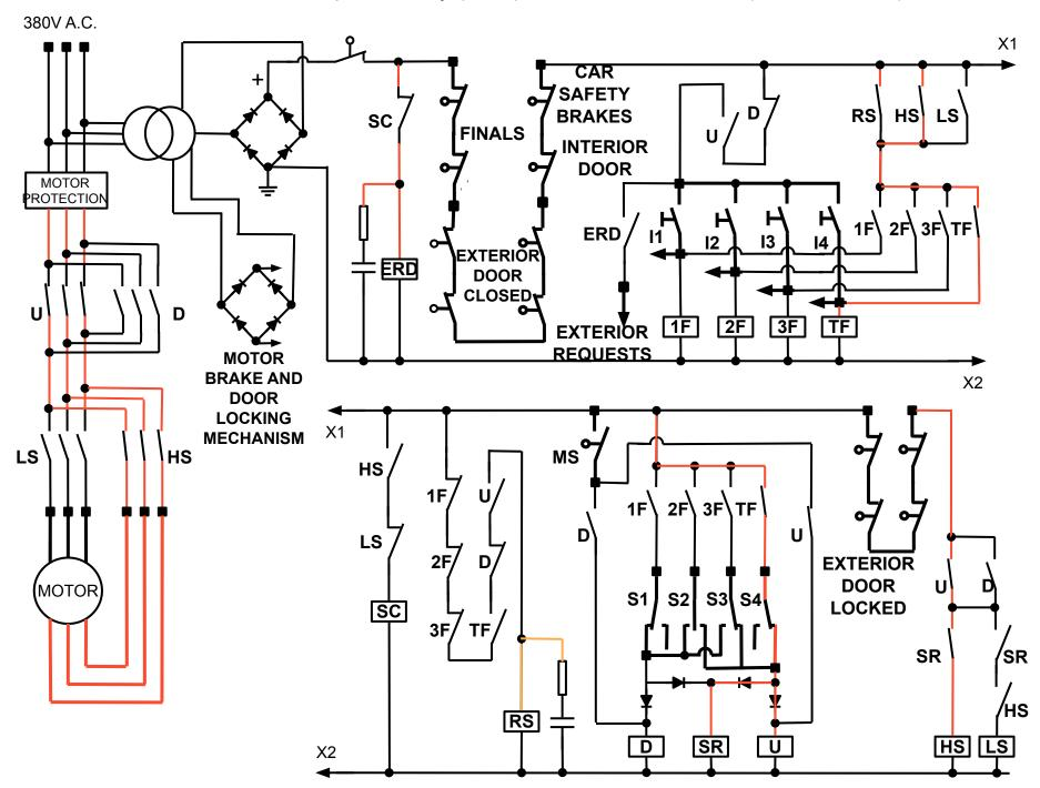
Since the car moves from the floor the level magnetic switch (MS) closes and the direction selector (S2) takes the down position
