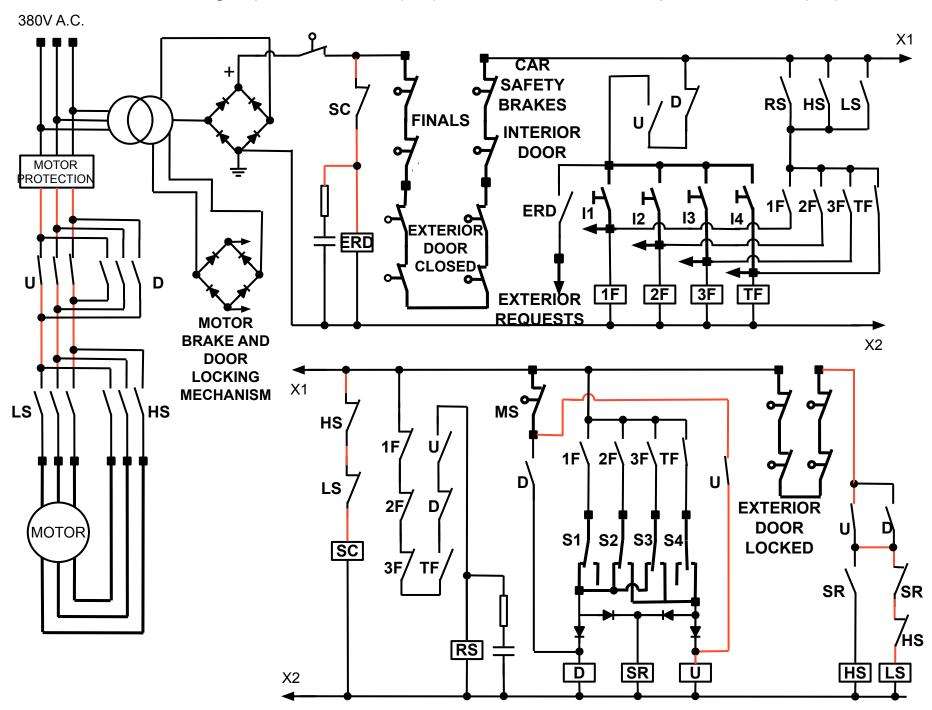
The high speed contactor (HS) turns off, then the low speed contactor (LS) turns on The request relay (TF) turns off
