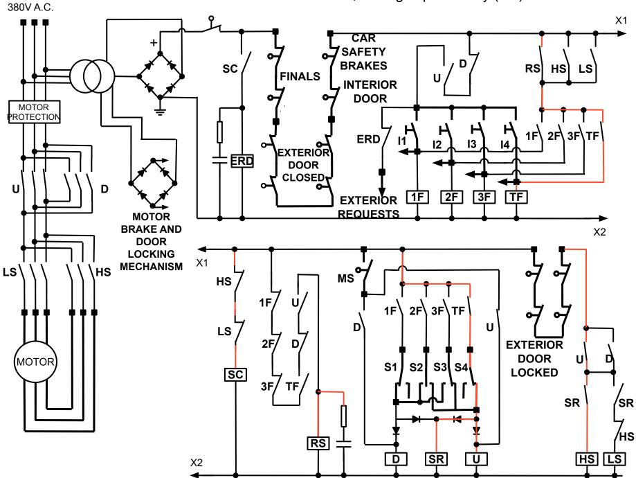
The direction contactor energizes the door locking mechanism. So, once the exterior door is locked, the high speed relay (HS) turns on and the car starts
