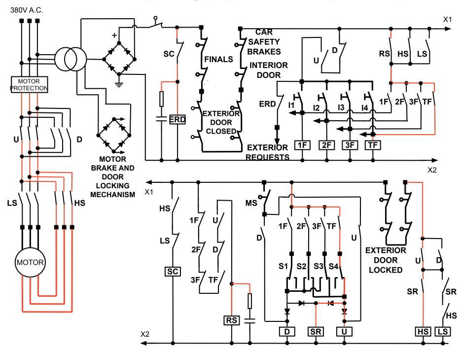
The exterior requests relay (ERD) turns on due to a NC (normal closed) contact of SC
