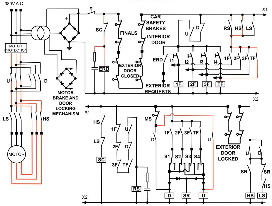
The high speed contactor (HS) turns off, then the low speed contactor (LS) turns on
