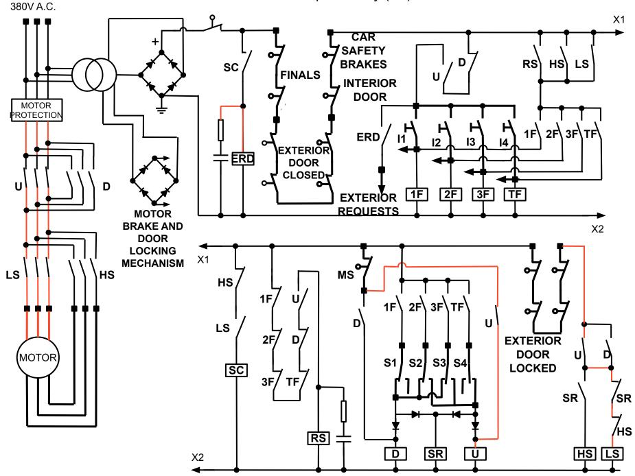
The high speed contactor (HS) turns off, then the low speed contactor (LS) turns on The request relay (TF) turns off
