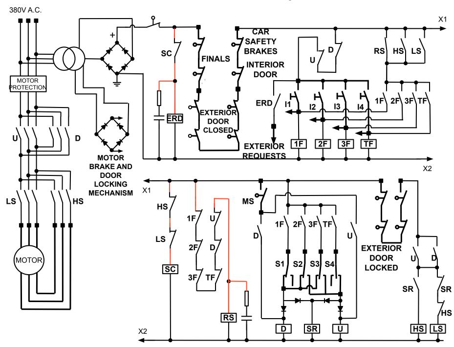
The exterior requests relay (ERD) turns off some seconds later due to the capacitor
