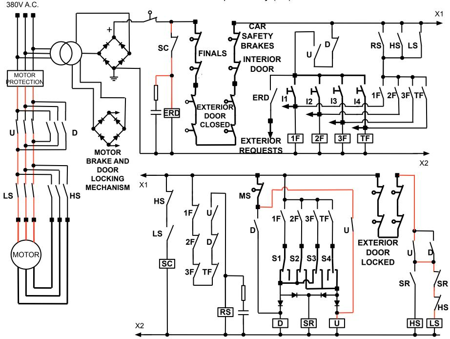
Once the elevator reaches the requested floor the level magnetic switch (MS) opens
