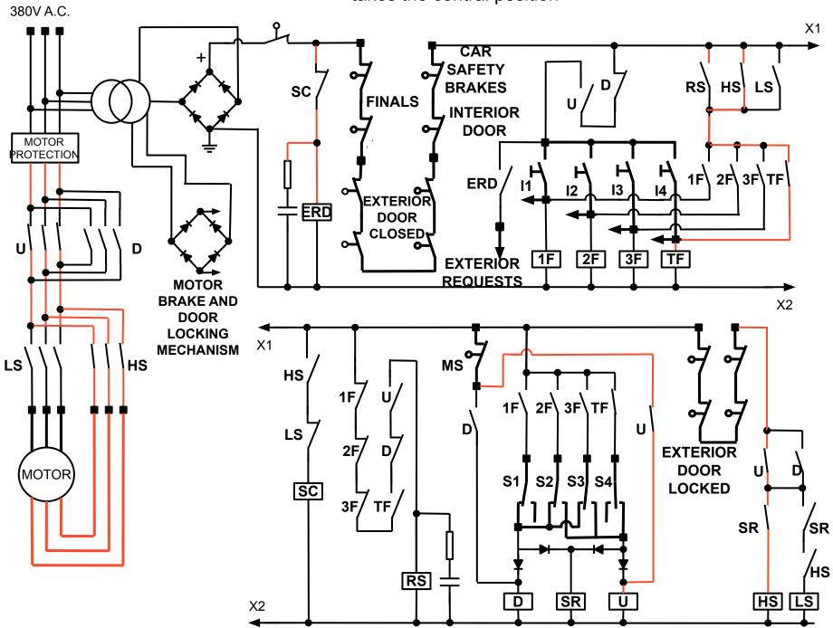
The direction contactor (U) is still energized, while the speed relay (SR) turns off due to the diode
