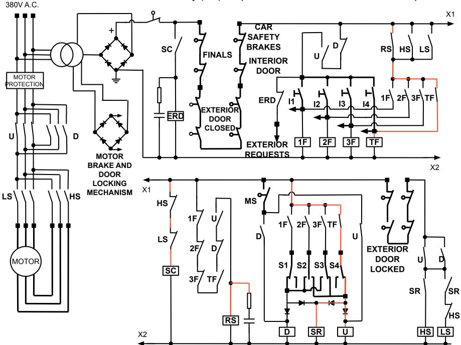
The direction contactor energizes the door locking mechanism. So, once the exterior door is locked, the high speed relay (HS) turns on
